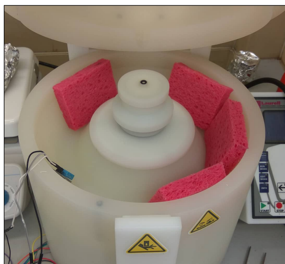
Spin coater containing warm, saturated sponges to alter humidity and a DHT11 humidity/temperature sensor
