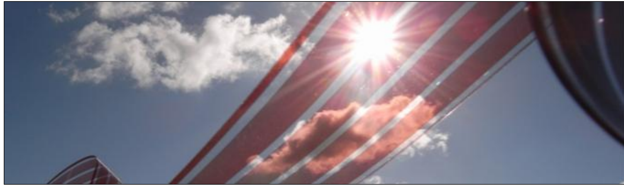
Flexible plastic solar cells created by Eight19
