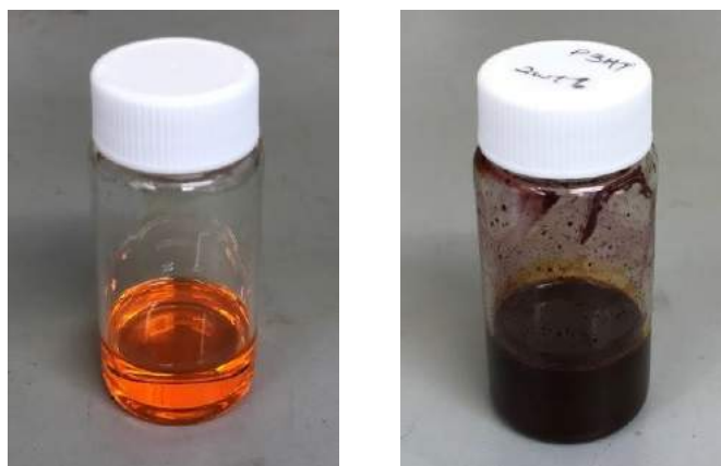
Figure 4.12: When P3HT is completely dissolved in p-xylene, the solution gives a bright orange colour (left). However, the colour of the solution changes with ageing to dark purple (right).
