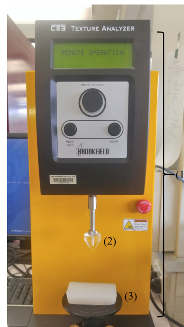
FIGURE 3.3: Equipment setup: (1) CT3 Texture Analyser, (2) conical probe and (3) hydrogel sample
