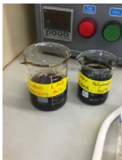
Figure 8: Precipitated PANI powder darkening beaker. Labels showing name, date and contents were essential to ensure safe laboratory processes.
