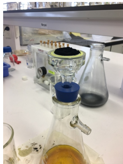
Figure 5: Thick layer of PEDOT powder sitting on vacuum pump filter following filtration. Spent yellow filtrate solution can be seen in the bottom of the flask.
