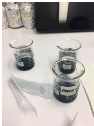
Figure 13: Beakers post-UV treatment, blue MB dye colour has disappeared to leave colourless solution with dark polymer powder.
