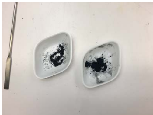
Figure 9: Synthesised PEDOT (left) and PANI (right) powders following drying and weighing of 20mg. Static on the weigh boats can be clearly seen. It was soon discovered that glass vials were much better than boats due to their lack of static electricity and better reliability of results.
