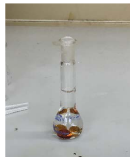
Figure 7: Aniline monomer in water prior to addition into diethylene glycol solution. Interestingly, aniline appears insoluble in water until the addition of the diethylene glycol and subsequent stirring, at which time the solution turns a light orange colour.
